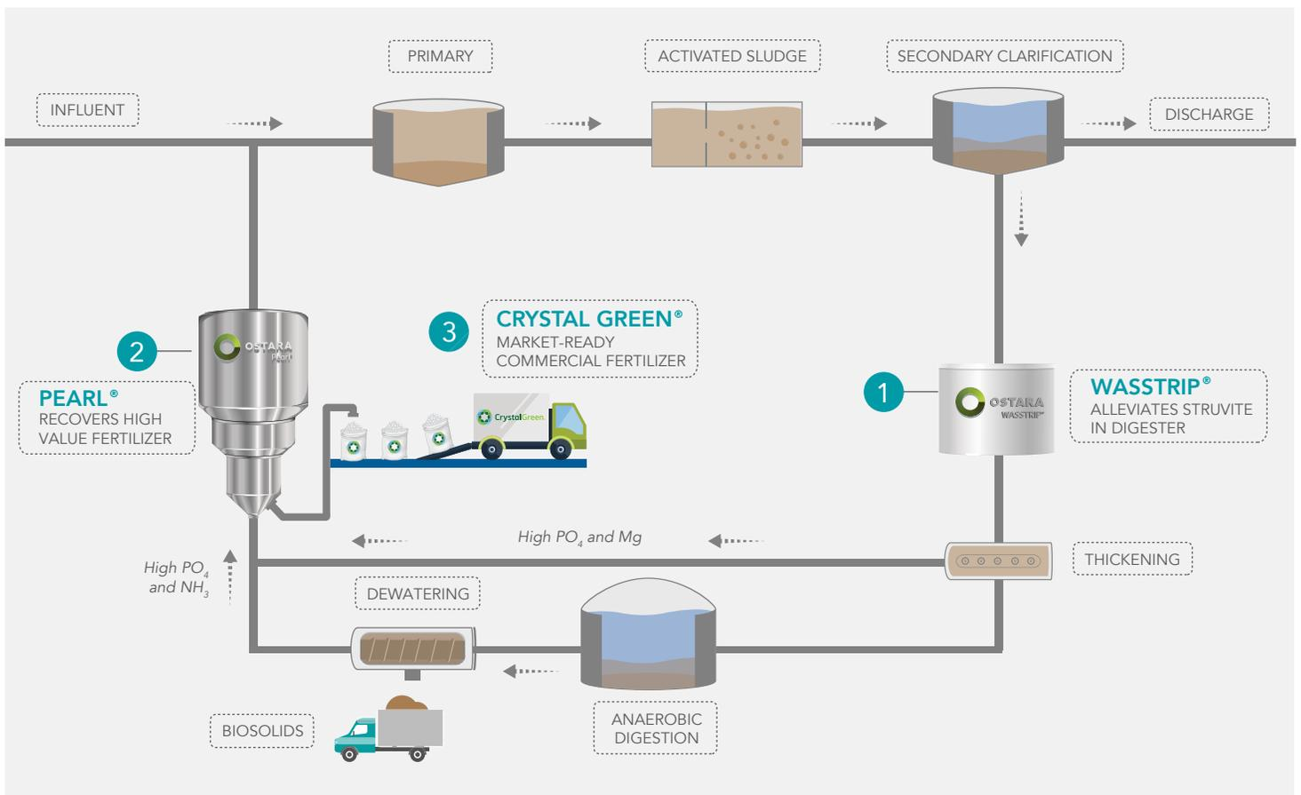
Figure 1 - Pearl® and WASSTRIP® solve operational challenges while optimizing phosphorus recovery
